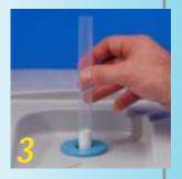
Insert sample into NMR chamber for analysis.
