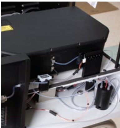
Hermetically sealed spectrometer eliminates frequent desiccant regeneration.
